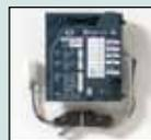
This acceptor will take up to 12 different coins, or tokens, and the value of any coin can be programmed in. Quarters are pre-programmed in switch #10 and dollar coins are in #11. Refer to the enclosed QL instruction manual for programming instructions if tokens or any other coins are to be accepted. **Do not unplug the QL from circuit board when programming, as it needs power to operate.**
