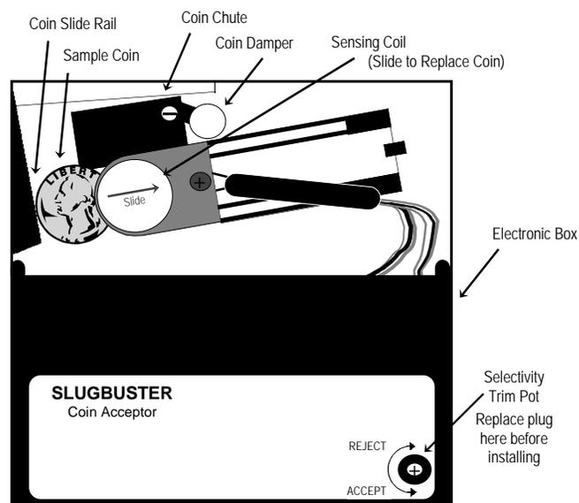
**Do not tamper with screws or nuts covered with blue sealer.**
