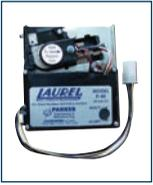
This acceptor sends one pulse to the LED display for every coin or token entered. The factory setting for the pulse value is \$0.25 but this can be changed if needed. To change, press and hold in the MODE button until the display reads; **SET PULSE VALUE**
