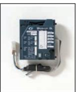
This acceptor will take up to 12 different coins, or tokens, and the value of any coin can be programmed in. Quarters are pre-programmed in switch #10 and dollar coins are in #11. Refer to the enclosed QL instruction manual for programming instructions if tokens or any other coins are to be accepted.
