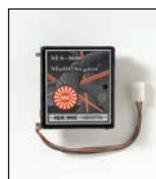
This acceptor will take up to 6 different coins, or tokens, and the value of any coin can be programmed in. Quarters are pre-programmed in switch #6 and dollar coins in #5. Refer to the enclosed MA850 instruction manual for programming instructions if tokens or any other coins are to be accepted.
